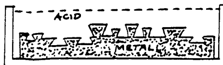
Diagonal undercutting can ruin work if left too long in the acid or solution too strong.
